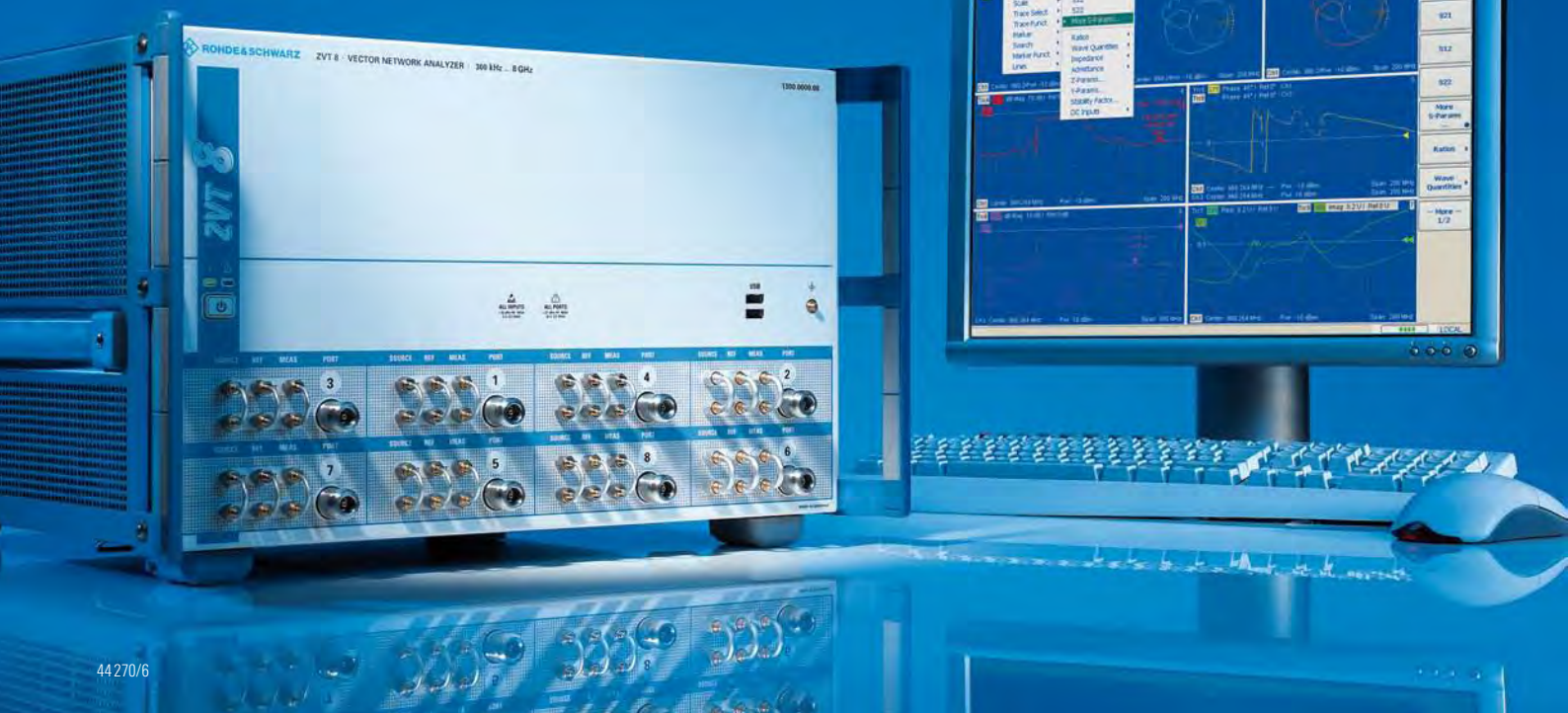
FIG 1 Vector Network Analyzer R&S®ZVT 8 – the world's first eight-port analyzer.
